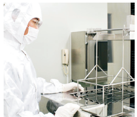
Ultrasonic Cleaning (Class 10000 Clean Room)
